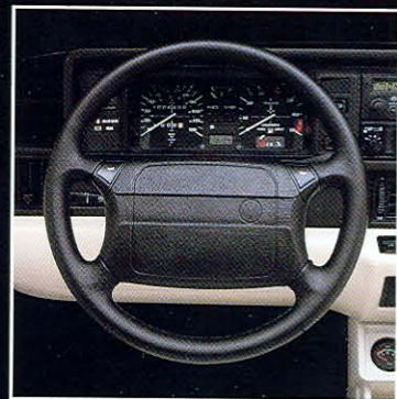
A leather-wrapped 4-spoke sport steering wheel with integral driver's side air bag is standard on Cabriolet Boutique.
