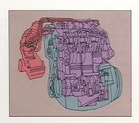
Cabriolet's CIS fuel-injection system features a precision fuel distributor and fuel metering valve to help maintain efficient fuel-air mix. An electric fuel pump and pressure regulator provide positive and uniform fuel supply and pressure.
