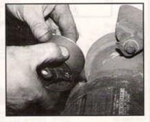
LEFT, the old mount must be cut, or pressed out from the carrier. Mesa West has a special tool that makes this chore a snap. ABOVE CENTER, our original right motor mount was totally collasped, even though the rubber looks great. ABOVE RIGHT, before pressing in the new motor mount, a chamfer is ground all the way around it to help center it.
