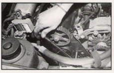
LEFT, once the belt is removed, the two bolts holding the mount carrier to the face of the engine are removed, as is the rear drive belt cover. RIGHT, the intermediate shaft sprocket must also be removed. To loosen the mounting bolt, use an extra 3/8-inch drive ratchet fitted with a long 13mm socket through the sprocket to keep it from spinning.
