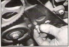
ABOVE, installation of the motor mount carrier is in reverse of its removal. The engine support jack may have to be raised, or lowered some to get all the screws in. Also, install all of the carrier's bolts before tightening any of them. ABOVE RIGHT, the timing belt is reinstalled by matching the paint markings that were put on before removal. RIGHT, the procedure is finished like a normal timing belt change from here.
