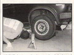
ABOVE, loosen the lower shock bolt and the wheel lug nuts, and raise the rear of the car. Place jack stands on the chassis, not the rear suspension axle beam or trailing arms. Remove wheel, the lower shock bolt, and the coil-over assembly.
