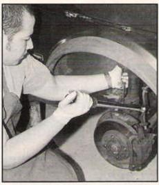
ABOVE, finish up the front by torquing both lower strut bolts/nuts to 59 ft.-lb., and reinserting the brake line in the strut's built-in holder. Add wheels, lower off jack stands, and torque lugs to 81 ft.-lb.
