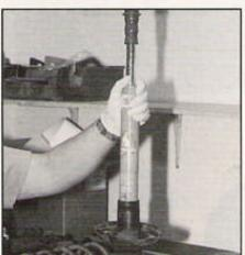
ABOVE LEFT, after removing the strut nut, and top components, slowly release the spring compressor from the spring, and remove it from the strut. Using a spanner wrench, large Channel-Locks, or a simple hammer and screwdriver (shown), loosen the stock strut gland nut and remove. ABOVE RIGHT, the stock shock uses the strut as the body, and is full of oil. Carefully remove the shock insert and drain shock oil.
