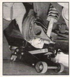
ABOVE, Adrian then used a floor jack to raise the trailing arm so the lower shock bolt would slip right in. Add the nut and torque to 33 ft.-lb. With the tire on, and the car on the ground, torque the upper nut to 23 ft.-lb. and replace the protective cap.
