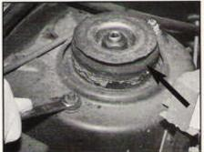
ABOVE LEFT, minutes after arriving at ABD Racing, ace mechanic Adrian Saldivar had the Cabriolet's chassis up on jack stands, removed the front tires, and got busy removing the two lower strut bolts from the wheel bearing housing. ABOVE RIGHT, under the hood, the two strut mount retaining nuts are removed. Check out how worn the rubber is on our original upper strut mounts (arrow). And this was after the load was taken off.
