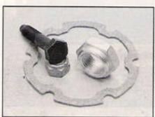
LEFT, in addition to the completely rebuilt drive axle assembly, you'll need to cruise over to the VW dealer and pick up a new axle nut, inner CV gasket, special "10.9" rated ball joint clamping bolt, and its mating nylock nut.
