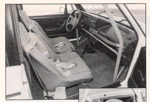
ABOVE, the dash is stock Rabbit except for a few slight modifications here and there. Note the Bug shifter and CB radio mounted to the tunnel. RIGHT, it's a whole new world under the front hood! 16-gallon fuel cell and ice chest fit neatly where the old powerplant once resided. Check out the PIAA driving lights behind the stock, late model Cabriolet front grille.
