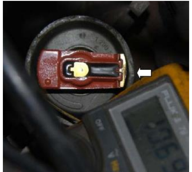
In this photo, the rotor tip has just lined up with the notch on the distributor body; the aperture is closed and voltage has gone HIGH. This is the moment the Hall generator signals the Hall control unit.
