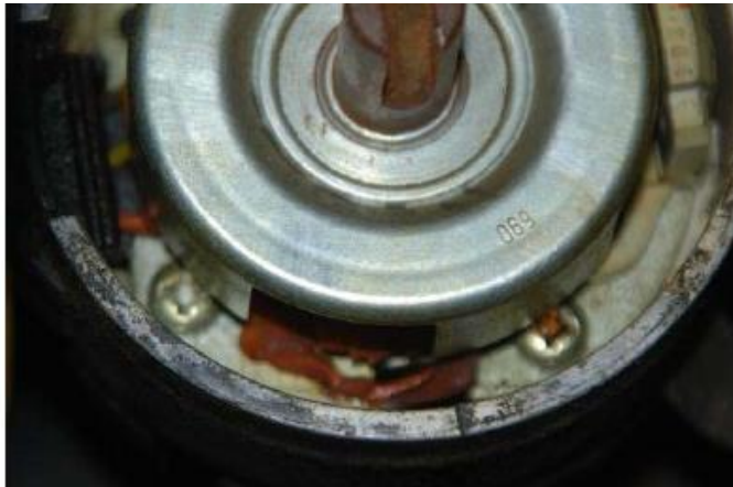
An old photo showing the shutter wheel position as the rotor lines up with the notch.
