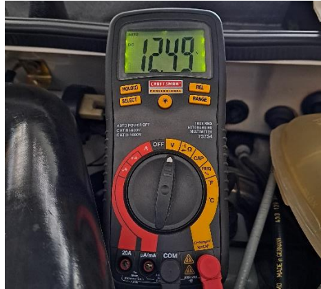
(This battery was actually 12.6V; the old meter pictured reads low.)
