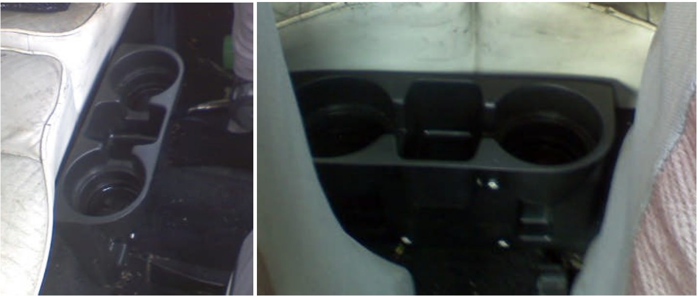
Mounting style: Screws or requires slight modification (as seen in photos). In photo, metal piece was added to the back, which is then slipped under the rear seat. Available at: Walmart and other parts stores. Various colors are available.
