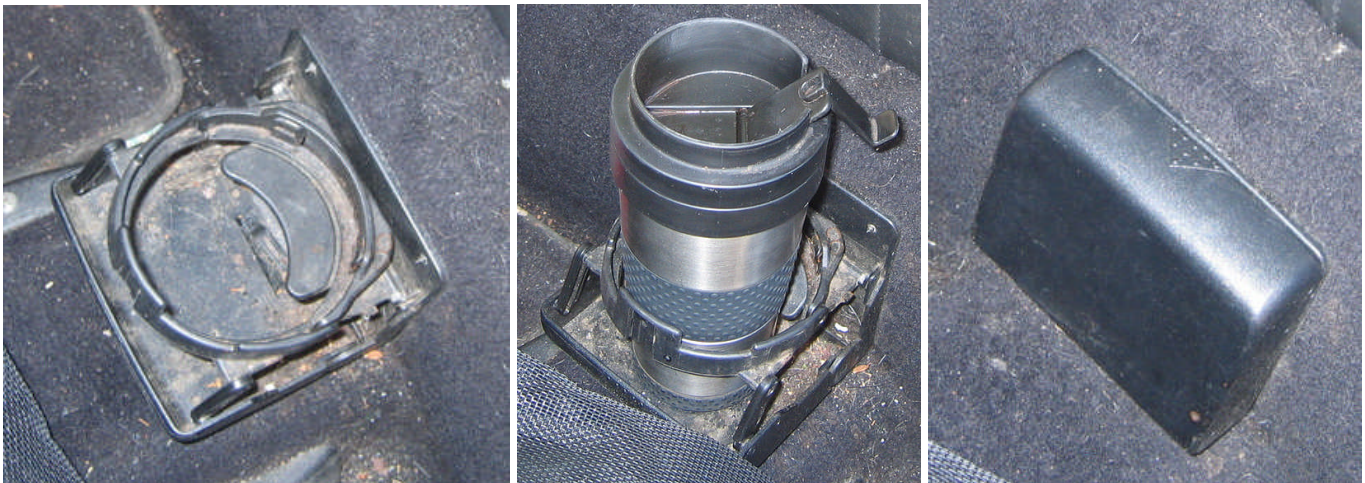
Mounting style: Screws or adhesive. In photos, mounted to center of rear seat platform at "hump". Available at: Most auto, boat and RV parts stores. Various colors are available.
