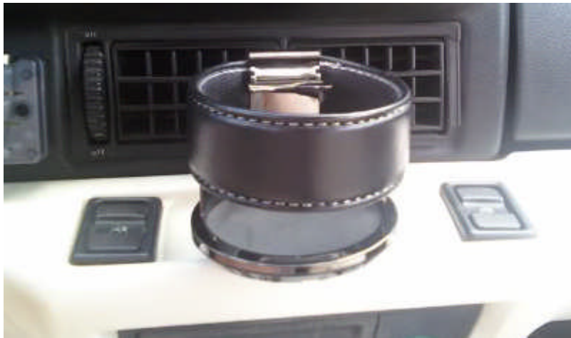
Mounting style: Clips to air vent, Velcro on the bottom. Available at: AutoZone or online stores (part #05597-8).
