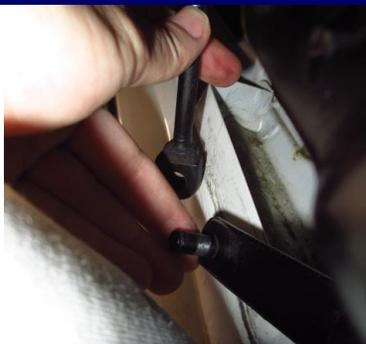
Pull the strut's lower-end off of its mounting post. Note: This post is mounted on a moveable arm.
