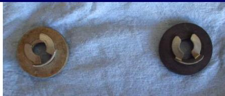
Install new strut (installation is reverse of removal), piston-end attaching to the bottom post (the one on the moveable arm). You may need push in on the washers in order to reinstall the circlips.
