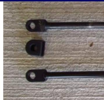
Remove the upper and lower rubber caps and place them onto each end of the new strut.
