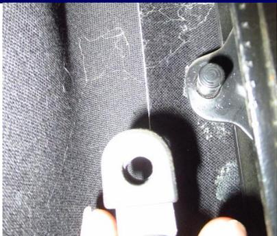
Pull the strut's upper-end off of its mounting post.
