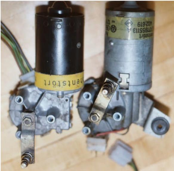
The 191 is mounted on my A1 car the same position as the 171 was: on the driver's side of the bracket. Three bolts. Better leave the harness plugged in the motor as you install it, making sure to clear the wires from the wiper drive linkage, because the connector will be in a hard place to get to if you have big hands.
