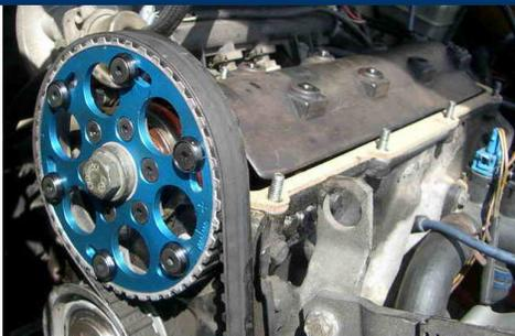
Install the new camshaft and cam gear. Installation of the new camshaft is the opposite of the uninstall. Make sure you use a lot of oil on the bearing caps and you install them in the order you removed them. Don't tighten one cap at a time, but tighten a little bit on each one evenly.
