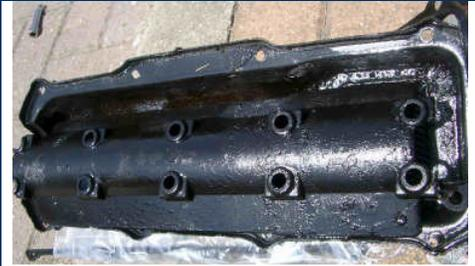
Thoroughly clean the valve cover and/or camshaft cover.
