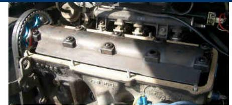
Install the new valve cover gasket (if you previously installed a rubber gasket, replacing it is not necessary unless the gasket is in poor shape).
