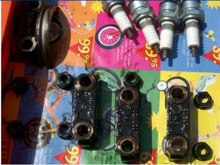
And now the most important part of the uninstall: The bearing caps. **Undo the nuts evenly an all 4 caps to avoid excessive pressure on one side of the cam.** When the caps are out, put them on a clean paper towel in the order they were removed. **THIS IS VERY IMPORTANT!** If you mix them you could have problems after. Here are mine. They go from left to right in the order that they appeared on the camshaft. I also kept the position of the nuts just to be safe.
