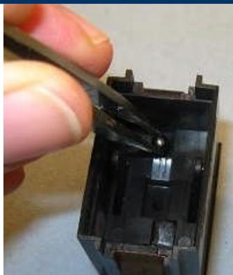
Reassemble. Remember the little metal ball? It goes back in the switch as pictured, at the indent at one end.
