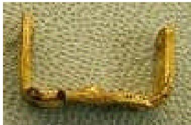
You're mostly concerned with the "spring loaded contact" component. Remove the U-shaped contact. It should slip right out. Be careful of the spring underneath it and the spring on the opposite side that pushes on the little metal ball. Both of these springs should sit freely in the hole, not binding. If either spring binds, or is damaged, you found your problem. Replace.
