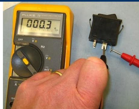
Test the switch to see if it works and that you bent the contacts enough. The meter should read infinite when the switch is off and less than an ohm when the switch is on. If not, go back in and bend/clean the contact a little more.
