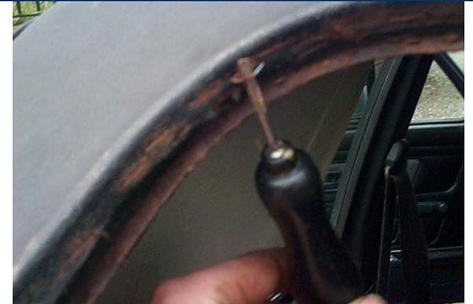
Now we have to remove the frame from the roof/top. Get a small screwdriver/knife and very carefully pull out the staples, there are a few. Be careful not to rip the top material.
