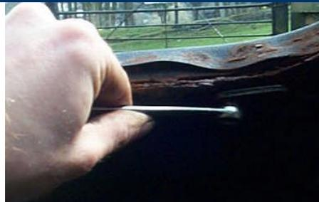
Undo the four 10mm bolts from the inside that hold the frame to the hinge.
