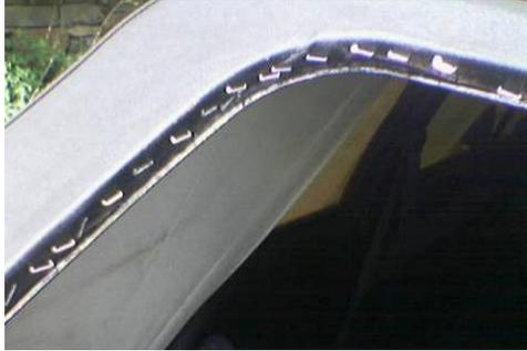
Get your new frame. You're now going to staple the new frame back in place. Starting at the top of the frame with the roof closed, you must match up where the old frame sat. Have some friends help you stretch the top material and staple it. The staple gun I used only pushed the staples in half way, so I just used a drift and hammer to knock them in all the way; some bent some went all the way in. Staple all the way around getting your helper(s) to pull the top material tight as you staple.
