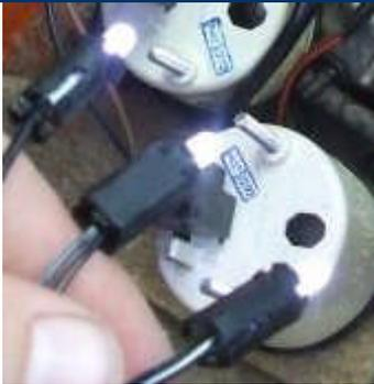
Carefully remove the original bulbs from each of their sockets and likewise with the LED bulbs. Insert the LED bulbs into the original bulb bases. (Some altering may have to be done to the bases.) Skip to Step 5.
