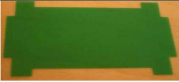
Once all 4 screws are out, you can lift the white cover and have access to the LCD screen. The LCD screen is held in place by two rubber pieces. Under the LCD screen you will find the green film that gives that nice green light; remove that film.
