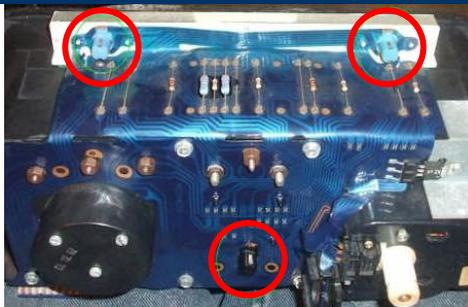
Lay the cluster on a table and remove (twist) the three original bulbs (locations circled).
