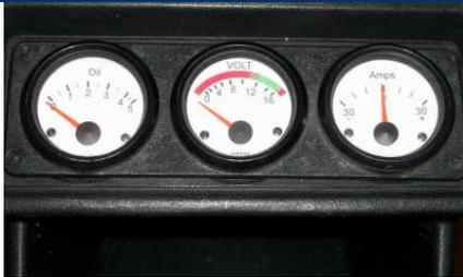
Remove the center console, the three VDO gauges, and the VDO bulbs.
