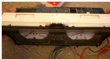
If you are changing the color of your cluster's lighting: Carefully remove the white cover from the top of the cluster, pull out the green film & reinstall the white cover.
