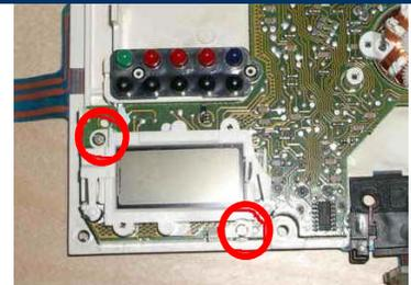
Now, you'll need to remove the screws holding the front and back cluster pieces together so that you can get to the inside. Once you get to the clock & idiot light circuit board, undo the two screws circled. There are another 2 screws under it. To undo them, lift the circuit just enough to get a small screwdriver in at an angle to get them out. You cannot get the board out unless you remove the flexible board completely. They are attached together.
