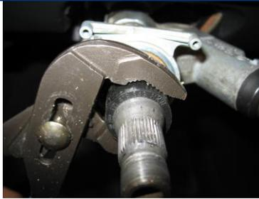
**Without airbag:** Using channel lock pliers, lightly grip the plastic spacer sleeve and "walk" the sleeve off the shaft using a back-and-forth-pulling motion (or rotate it counterclockwise while pulling).
