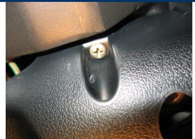
Using Phillips screwdriver, remove the two steering column cover screws, and remove lower cover.
