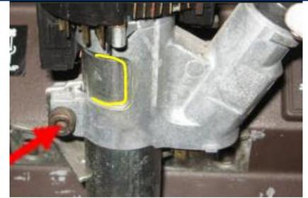
Using a marker, mark the location of the switch housing on the steering column (yellow line in photo) so that you can reinstall it in the exact same position.
