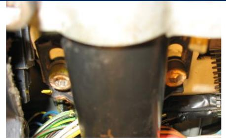
Remove the upper steering column cover. This may require loosening the 4 steering column Allen screws so that you can push down a bit to free the upper cover.
