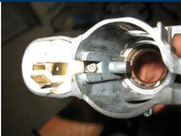
Using Phillips screwdriver, remove screw and switch.
