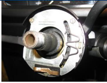
Using flathead screwdriver, remove the 3 retaining screws for the turn and wiper stalks. Remove the two stalks.
