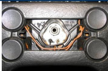
**Without airbag:** Remove center pad by carefully prying it out with a small screwdriver or interior removal tool (1983-1987 sports wheel shown; others are similar). Disconnect wires, if need be.
