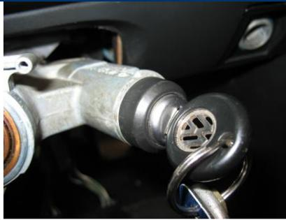
Put the ignition key into the ignition lock/switch cylinder and put in "on" position.
