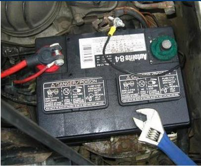
Using 10mm wrench, disconnect battery negative terminal.
