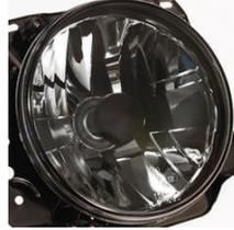
Headlamps that have no lens optics. They come in both 7" and 5" sizes and are also available smoked. These lamps usually use the H4 and H3 bulbs listed above and, aside from a wattage upgrade from the stock sealed beams, these headlamps are cosmetic replacements and are usually not street-legal.
