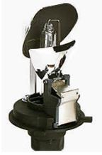
HID stands for high-intensity discharge. Rather than a glowing filament, this type of lamp produces light by an electric spark arcing across a gap inside a Xenon gas-filled capsule. This type of lamp produces a brighter, truer-white beam of light. Very expensive type of headlamp. These bulbs also cause glare problems for oncoming drivers because HID bulbs are designed for use in projector housings. These bulbs should not be installed in standard H4/9003/HB2 headlamps!
