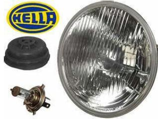
A 7" round headlamp and dual-filament bulb assembly that looks like a sealed-beam headlamp that uses a replaceable H4 or 9003/HB2 bulb. The H4s came standard on European cars (see E-code below). The 9003/HB2 is the DOT's version of the H4, but these were never installed on the cars at the factory. The two bulb types are slightly different: the H4 is designed for E-codes, while the 9003/HB2 bulbs are designed for DOT. All, however, use the same socket pattern.
