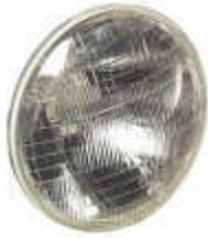
A 7" round Halogen, dual-filament sealed-beam headlamp with lens optics that came stock on Cabriolets sold in North America. These headlamps are usually marked with "DOT" on the lens. If your Cabriolet has the dual-round set-up, these headlamps are the *outer* lights and are both hi- and lo-beam.
