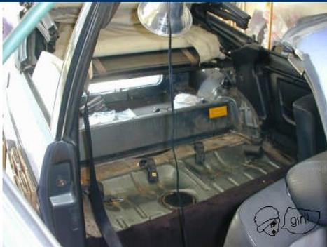
Remove the rear seatback by unscrewing the two screws at the base of it. Open your boot and pull the release button, and then the release cord. This is a bit of a maneuver, but by lifting and pulling, the seatback will come out. Set it aside.
