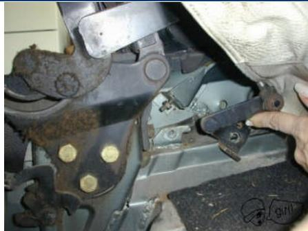
Remove the gas shock bolt. Remove the perpendicular bolt. Take the nut off the rear tension cable.
