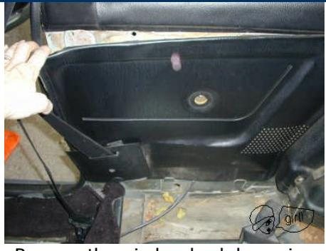
Remove the window knob by prying up the cover and unscrewing it. This is in the Haynes and Bentley. Remove the interior card by pulling the door trim away from the edge and prying the fasteners loose. They will pop out. The seat belt trim may have a little holding knockout that will have to be pried up.
