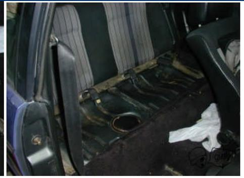
Remove the rear seat by unscrewing the two screws that hold it down. These are right in front of it. Bag the screws and label the bag. Bag and label every screw or other fastener you remove. There will be lots of them. Slide the seat bench forward and pull it out. Set it aside.
