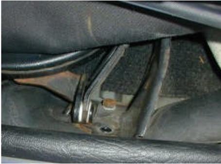
Next step could be done before, but I didn't think about it. Duh. You now have to free the window frame hinges and the rear headliner tabs. Pull the top up at the back and look for the hinge mounts. Each has two bolts. Remove the bolts. The itty bitty wrench is your friend for the bottom one. If you did this while the top was still on the car, you could probably reach both with a socket.
