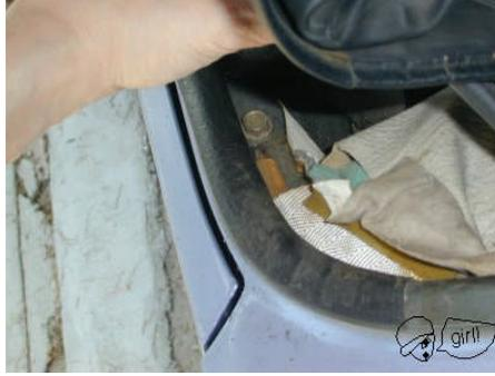
The rear headliner tabs are secured with a fitting that is screwed and bolted into place. One screw and three bolts. You can see the screw and one bolt here.
