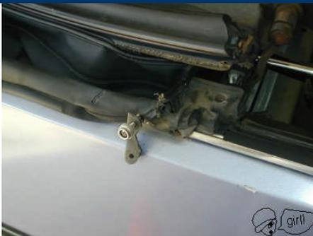
Get out of the car and remove the screws from the [caps] where the boot snaps on.
