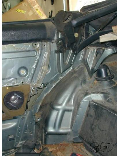
With the bolster trim out, look carefully at the frame mounting. The top should be fully down but released at this time. Note which bolt is visible and mark it with the pen.
