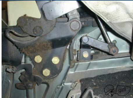
Study the frame mounting. You will see a cluster of 3 bolts, a fourth bolt holding the gas [strut], and a fifth bolt perpendicular to those two. If you look carefully, you will also see the end of the rear cable for the top.
