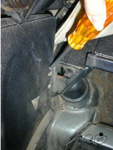
If you follow the curve of the bolster, you will see two more screws that would be hidden by the seatback. Remove those two screws. Pull the top release handle off its lever. Remove the bolster trim.
