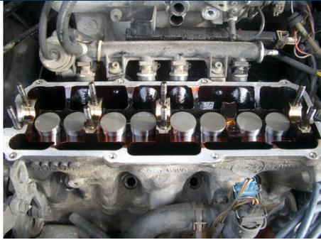
Remove the valve cover and camshaft.
