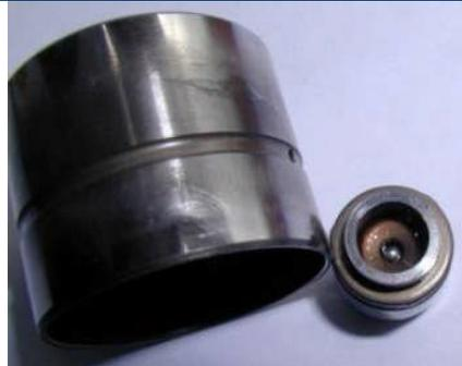
Again, fully clean out the inside of the tappet, getting rid of any oil deposits, gum varnish etc. This is done by using a small brush/Q-tips with some Gunk poured onto it.
