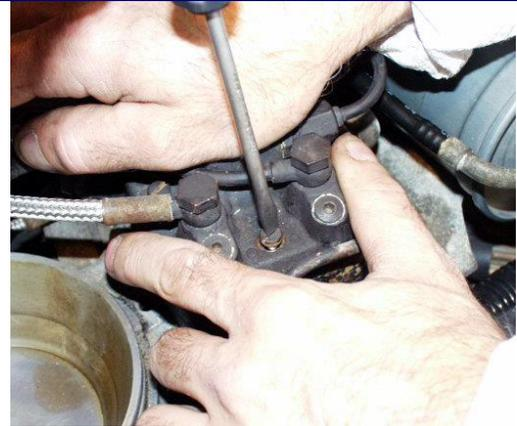
There are three flat head screws (the engine side one might require to loosen an injector line and move it temporarily) remove the screws.
