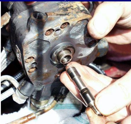
Slide the plunger out gently, until the soft return spring comes out with it. Remove both from the unit. Using a soft cotton ear-swab dipped in gasoline, clean out the residues inside the injector body shaft.
