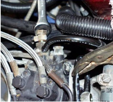
Next to the line you just closed, a line leads to the firewall side of the injection system. Gently crack the line open, and save the bolt and washer.
