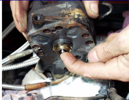
Gently pushing on the plunger, you will feel (and see) if there is debris inside the shaft (it should move up and down smoothly, without having to pull on the tip to make it come back in place).
