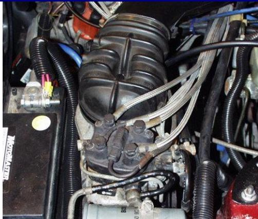
This is the fuel distributor. The valve is in the part with the fuel lines connected to it.
