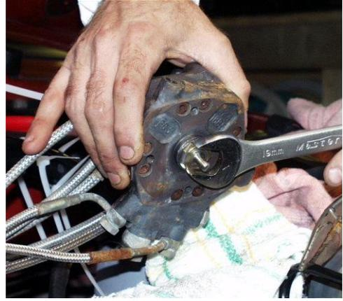
Slide the spring back into the injection assembly followed with the plunger making sure you have wiped the plunger with fuel first. Set the limiter ring in its original place and hand screw the nut back in place, tighten it down.
