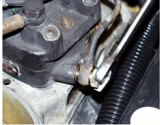
Lastly, on the battery side of the injection system, one last line you need to crack open, and remove the bolt and washer.
