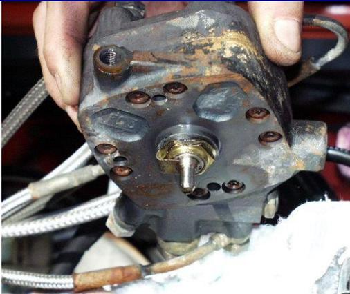
Gently lift the injection assembly from the airflow box. The plunger should be partially visible as it sits, resting on the edge of the travel limiter ring.
