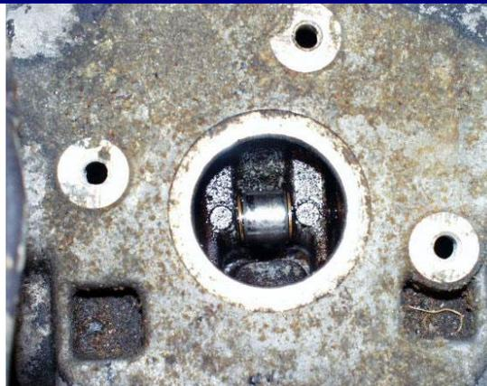
Here is a reason why you should NOT use carburetor cleaner to spray under the air box to clean it out – it collects stuff if improperly rinsed out afterwards. Clean it by hand with a cloth dampened with fuel.
