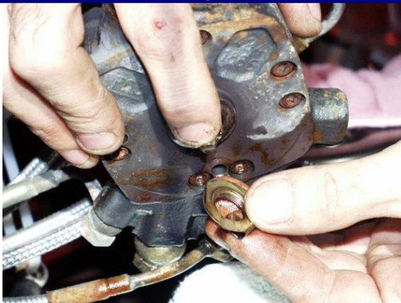
Loosen and remove the bolt and travel limiter ring, holding the tip of the plunger gently in place ~ do not use excessive force to hold it in position **(IMPORTANT! see why below!)**.
