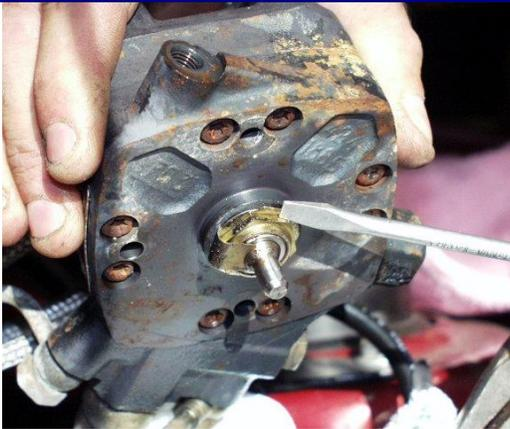
Right below the tip of the screwdriver is a lip, preventing the bottom from coming loose; you will need to flatten this upwards to remove the nut of this assembly. At this point, before going to the next step, you should mark on the body where the travel limiter ring position is, as you will need to return it into the same position when reassembling.
