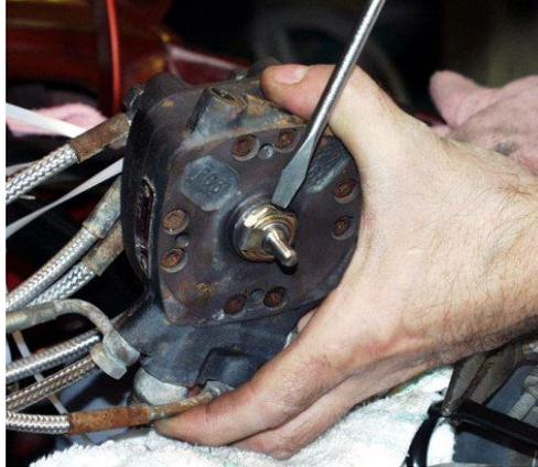
Don't forget to push the locking flap back in place, to gently put the injection system back on the airflow box, screwing evenly the flathead screws back in. Then reconnect the 3 gas lines to the unit, check for leaks, release the fuel line. Try to start the car, it WILL take a few turns of the engine to start – until the air has escaped the system, it will be a rough idle, but it should settle down inside of 3 to 5 minutes.
