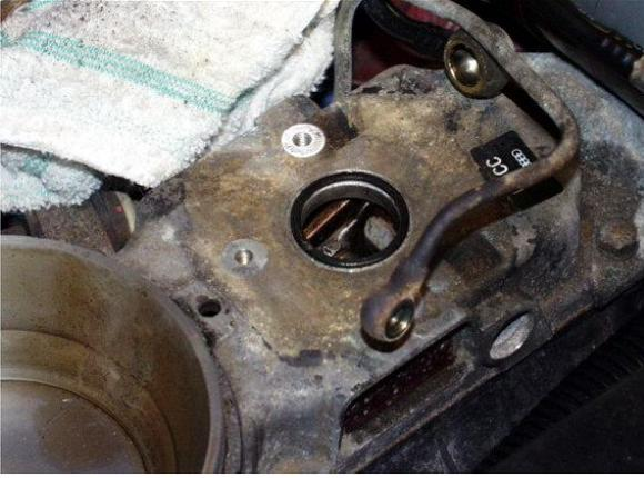
All Done. I finished by sanding evenly the 3 rest points of the injection assembly so that the plunger would be at the optimal angle of action once re-assembled.
