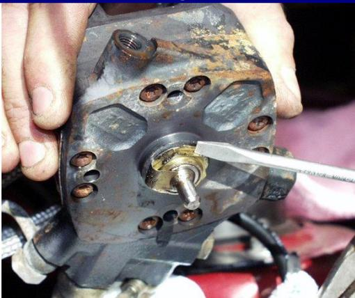
Right below the tip of the screwdriver is a lip, preventing the bottom from coming loose; you will need to flatten this upwards to remove the nut of this assembly. At this point, before going to the next step, you should mark on the body where the travel limiter ring position is, as you will need to return it into the same position when reassembling.
