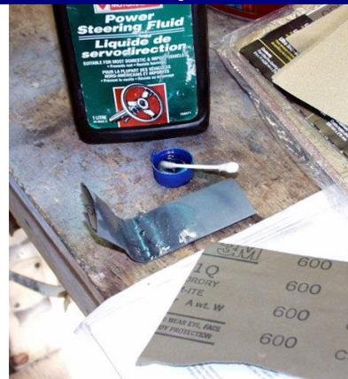
I noted a few scratches that were probably my cause for idle hesitation on the plunger. Using 600 grit sandpaper, and using a wetting agent (in this case power steering oil), I gently sanded the scratches from the shaft of the plunger until it returned to the original shining metal it was supposed to be. Patience and gentleness is important as this part cannot be purchased separate from the injection unit (which is a mere \$850 in itself).
