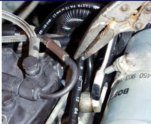
Using a pair of Vise Grips ("long nose" style), gently squeeze the tubing coming from the fuel filter to the injection system. DO NOT pinch the line, you only need as much pressure as to prevent gas from pouring out. Below it is a bolt; crack it open, remove bolt and copper washer.
