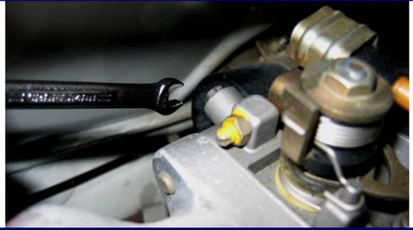
6. If the idle boost valve kicks in while you are adjusting, you've dropped too low on idle RPM. You can unplug the idle boost valve electrical connector, or better, pinch off either of the hoses going to it. When the idle boost valve (or hose) is reconnected, idle should not change if you've adjusted the idle correctly.
