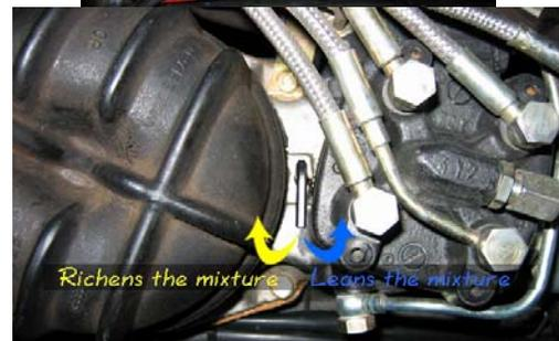
5. Have your 7mm open-end wrench handy; you may have to tweak the idle bypass screw (backside of the throttle body) if the idle changes too much. You need to stay below about 900 RPM while adjusting the idle. Use the tach on the dash and your ears, you know what sounds right and normal. If you go over 900 RPM, the centrifugal advance starts to kick in, changing the timing and confusing all your readings. Set the idle RPM at  $900 \pm$  but above the threshold of the idle boost valve.
