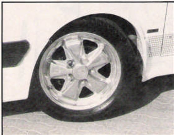
LEFT — For tires and wheels Chris used Porsche 912 15x5½-inch rims on the front and Porsche 356 deep spoke alloys along with 15x6 Fulda 195-50 series tires on the front and rear.
