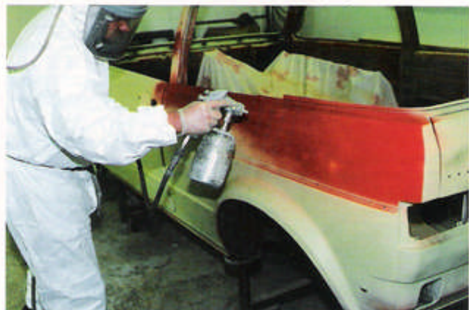
Paint is applied in two stages. Primer first, then the two-pack top coat.
