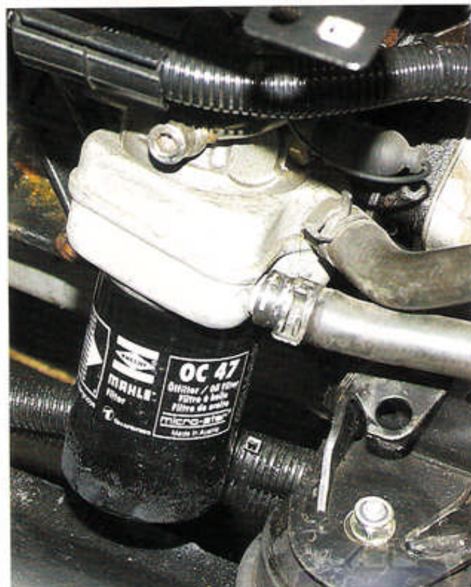
An oil cooler is often the biggest culprit when it comes to oil contamination
