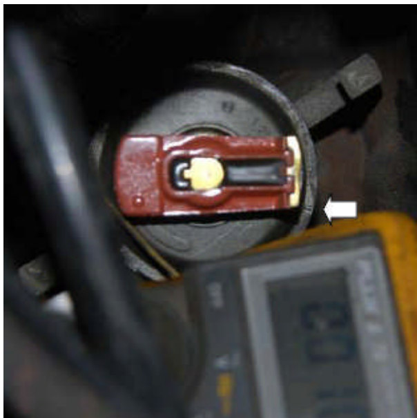
In this first photo, the rotor, turning clockwise, is approaching the #1 timing notch on the distributor body (white arrow); the shutter aperture is open in this position and voltage on the green/white wire is LOW.
