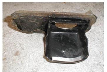
Here's a side shot of the shifter gate. The shifter goes in the hole, and you make out the stop just at the bottom of the photo. The part is removed from the car FROM THE TOP.
