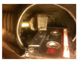
The thick part (head) is the proper size for the adjustment. Pin it in the lockout, and then tighten the bolt at the other end of the shaft that you loosened earlier. Put the car on the ground and drive away!
