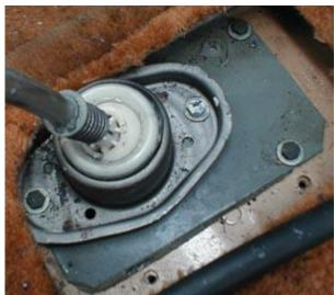
This is the top view of the shift gate installed. It's the square, gray metal plate bolted to the body of the car, underneath the shifter.
